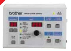
The minimum number of keys that are necessary for normal sewing operations are located on the simplified operation panel, along with an easy-to-see LED display. The operator can position the operation panel where it is most convenient to use.
