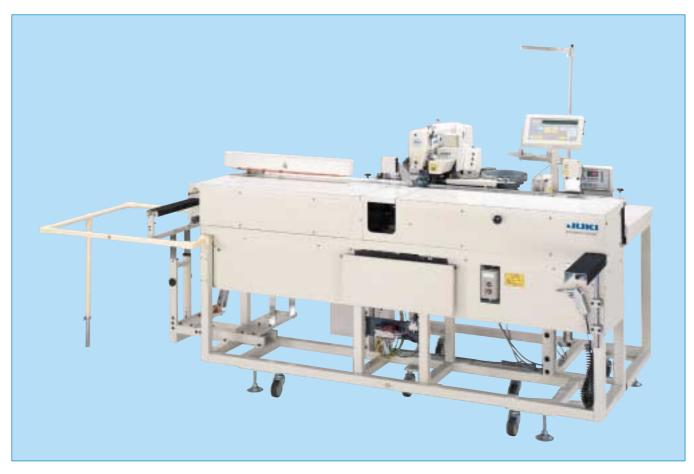
The machine is more productive and accurate than any of its predecessors. It responds more flexibly than ever before to the sewing of buttons on ladies' wear, finished products, and long-sized garments.
