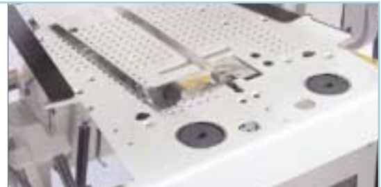
Maintenance works are conducted with the machine head tilted.
