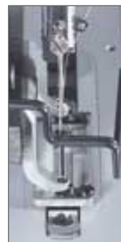
Position of the needle bar during sewing
