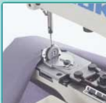
For sewing wrapped-around buttons (2nd process) *
