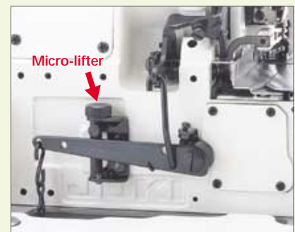
Bottom and top differential-feed micro adjustment mechanism
